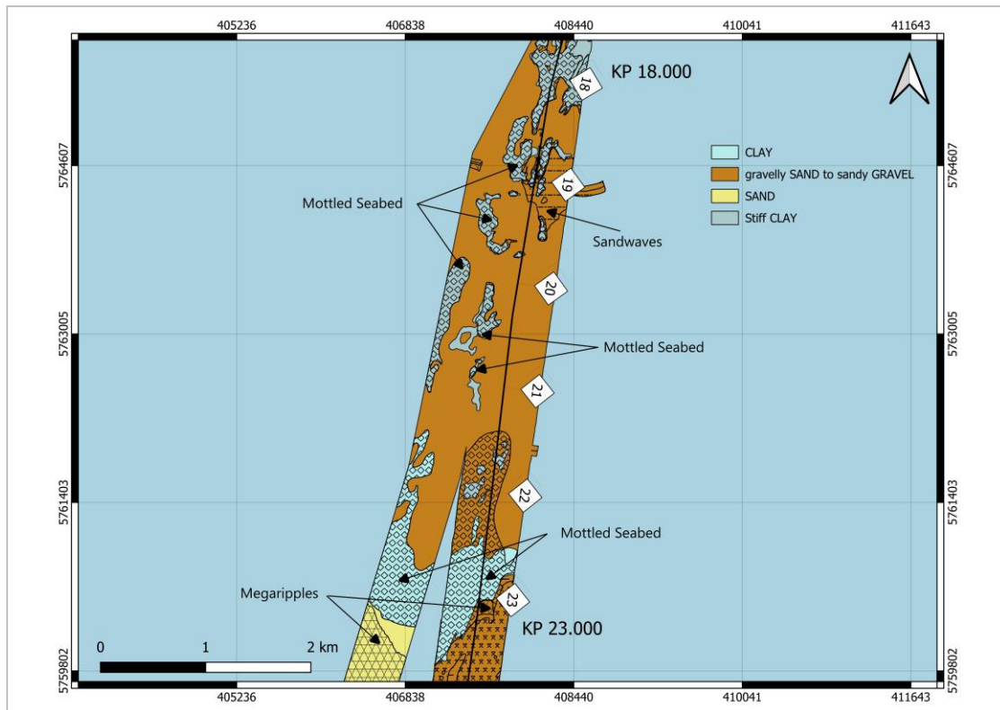
Figure 10-23: Overview of Seabed Geology and Features Block 2 between KP 18.000 and KP 23.000
