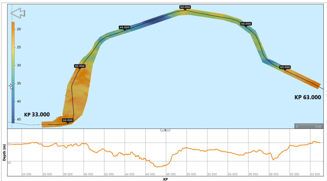
Figure 10-31: Overview of the Bathymetry in Block 03 between KP 33.000 and KP 63.000
