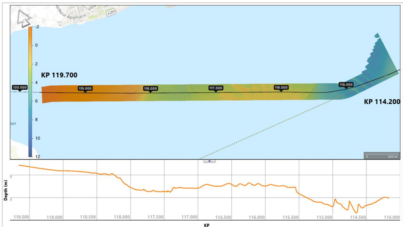
Figure 10-73: Overview of the Bathymetry in Block 05 Nearshore KP 114.200 to KP 119.700
