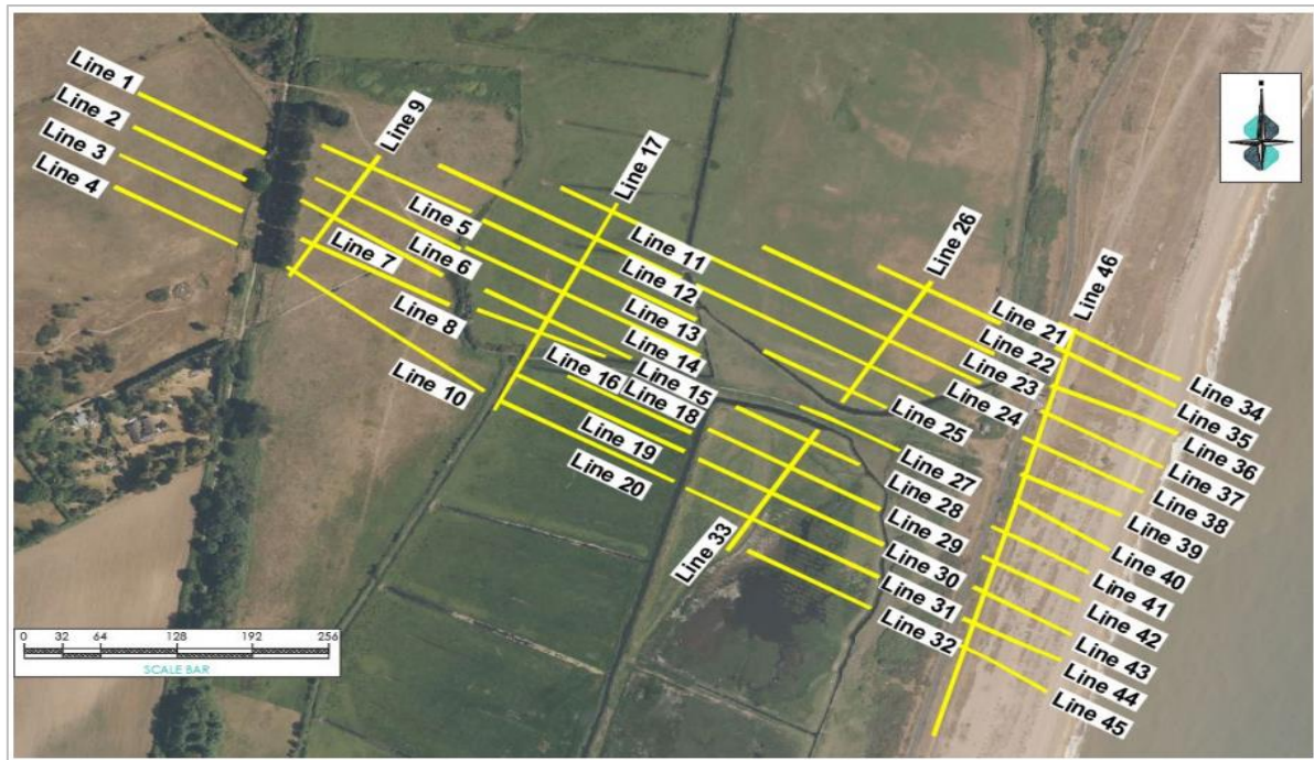
Figure 10-4: Seismic Refraction Survey Lines at Aldeburgh – Plan View
